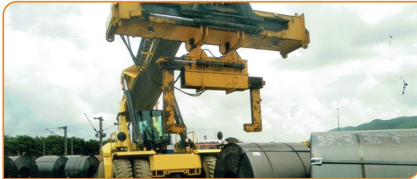
Coil Handling tong system suitable for any reach stackers
